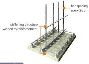
Upper reinforcement installation and welding to vertical bars.
